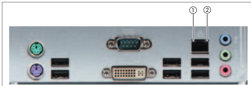
Figure 163: Indicators on the connector panel: LAN indicators
